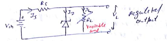
> The load resistance Re decreases, the load current increases This cause rener divele current to decrease, due to they inflid current Is & doop across the imput peristance remains Constant. Therefore the load valleage ve is also constant > How the load resistance Re, increases, the load current dercreases. Due to this rener current increase > This again keeps the values of expect current the vallage dup across suives resistance as constant. > Therefore, the load vallage remound constant.
